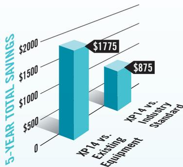
SEER stands for "Seasonal Energy Efficiency Ratio" and is a measure of the cooling efficiency of heat pumps. The higher the SEER, the greater your energy savings. Typical SEER ratings start at 13.00, but the XP14 carries ratings as high as 16.50. HSPF stands for "Heating Seasonal Performance Factor" and is a measure of the heating efficiency of heat pumps.
